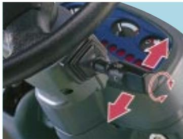
**Combination switch for head lamp and directional indicator (Auto-return)**
